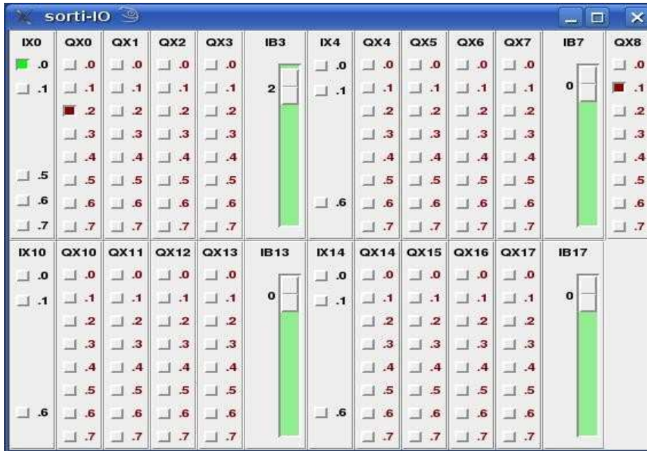
Fig. 3 iCbox as IO for “ sorti ”- IX0.0, QX0.2 and QX8.1 are “on”- the rest are “off”.
